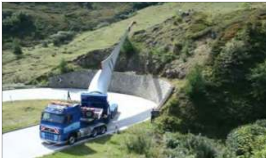
Plate 4-4 Blade adaptor transport system
